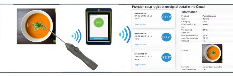
**Innovative solution:** with a built-in temperature meter and an unique BLUETOOTH SENSOR you automatically register product measurements and store everything directly online in your own digital folder.
