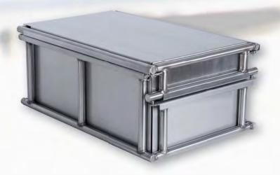
The PhoenixTM TS12 Series Oil Quench System (Patent Pending GB1509136.6), uses a multi-channel, high temperature data logger protected by a thermal barrier which uses a two part insulation system. The inner thermal barrier is completely sealed to prevent oil contaminating the data logger.
