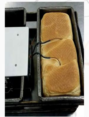
A range of thermal barriers is also available for higher temperture baking processes. Special designs are also available to meet individual customer application requirements.
