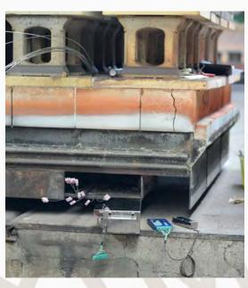
PhoenixTM systems are also available for roller hearth kilns. The system runs through the firing zone with the product and can measure both product and air temperatures.
