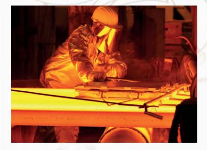
The TS07-100 Thermal Barrier System is specifically designed for Mini-Mill (CSP) applications. It provides thermal protection for the data logger combined with a support arm for the thermocouples measuring both surface and atmosphere temperature. After preparation the system is lowered onto the moving slab using the foldable suspension arms by an overhead crane. When positioned on the slab the arms are lowered to ensure the low height profile of the system is maintained.
