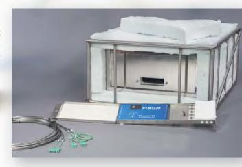
Developed from many years of experience the TS07 has many features specifically for this harsh environment. The data logger fits into an inner tray providing extra protection for the connections whilst clamping thermocouples to ease handling.
