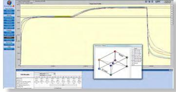
A separate software package, "Thermal View Survey" is available for surveying furnaces to AMS2750 requirements. Featuring thermocouple and data logger correction factors, user defined TUS levels and tolerances, View Frame analysis, overshoot search, data import / export, printed AMS2750 report. Contact us for a demo version!
