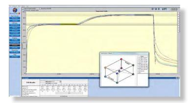
A separate software package, "Thermal View Survey" is available for surveying furnaces to AMS2750 requirements. Featuring thermocouple and data logger correction factors, user defined TUS levels and tolerances, View Frame analysis, overshoot search, data import / export, printed AMS2750 report. Contact us for a demo version!
