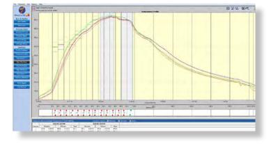
Comprehensive analysis tools are located on the left side of the screen for single click analysis and report generation. Data import and export in both .csv and PhoenixTM formats are available allowing electronic transfer of process data.
