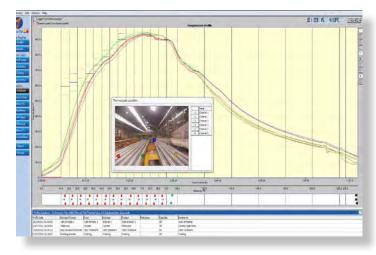
The temperature profile is displayed in the graphics window of the Thermal View software. Thermocouple profiles can be switched on or off individually and you can zoom in for more detailed analysis.
